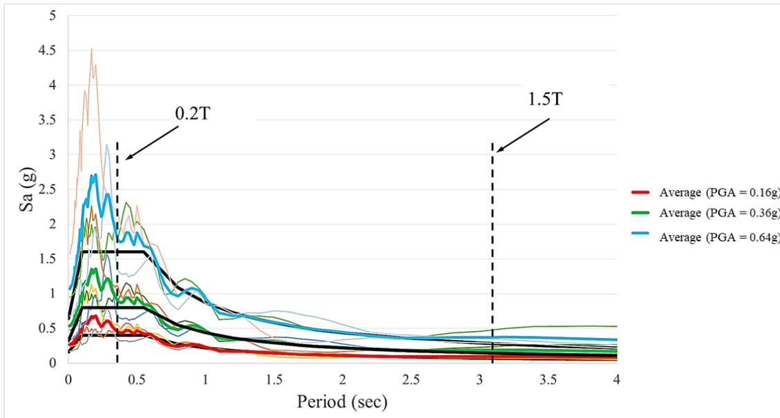
Figure 5. Response spectrum and the median response spectra of the three ground motion records for three hazard levels: (i) PGA = 0.16 g, (ii) PGA = 0.36 g, (iii) PGA = 0.64 g
