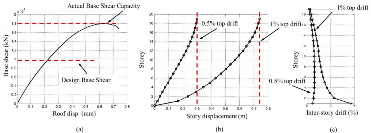
Figure 3. Pushover analysis results: (a) base shear vs. roof displacement, (b) storey displacement, (c) inter-storey drift ratio
