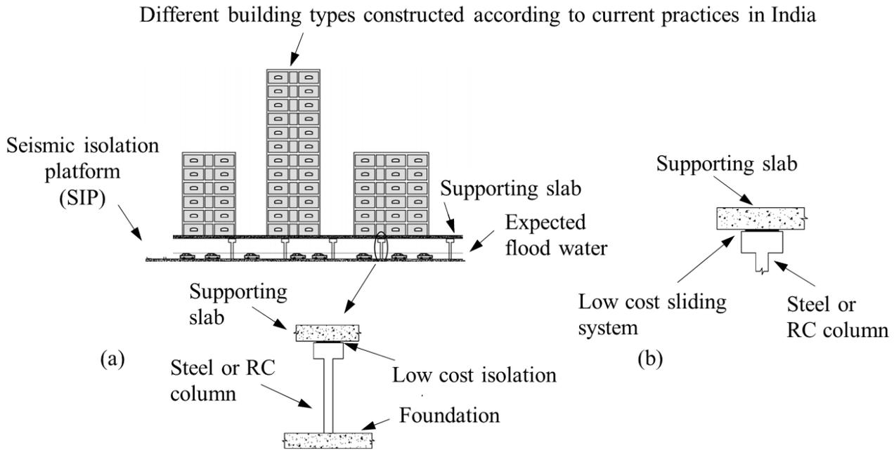
Figure 1. Resilient Seismic isolation platform (SIP) concept built to support buildings: (a) overview, (b) alternative low-cost isolation systems
