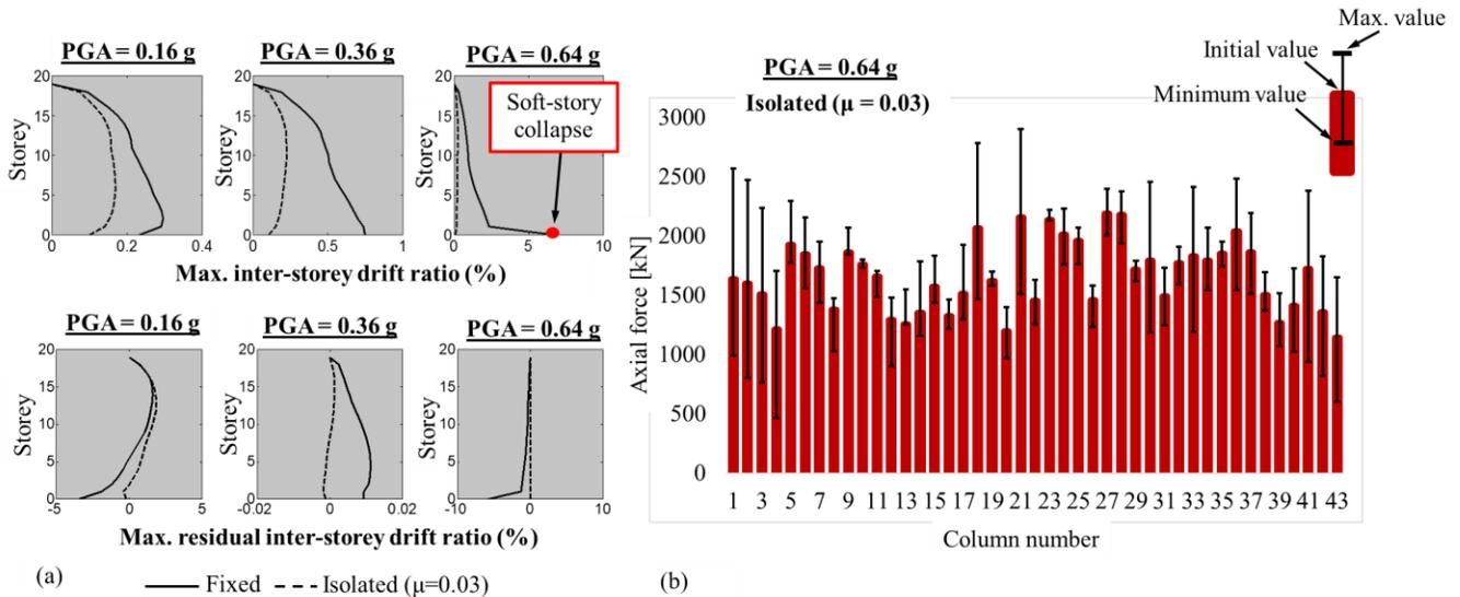
Figure 6. (a) peak global responses resulted from nonlinear response history analysis at three Peak Ground Accelerations, (b) average value of first floor columns' axial load variations for the isolated structure
